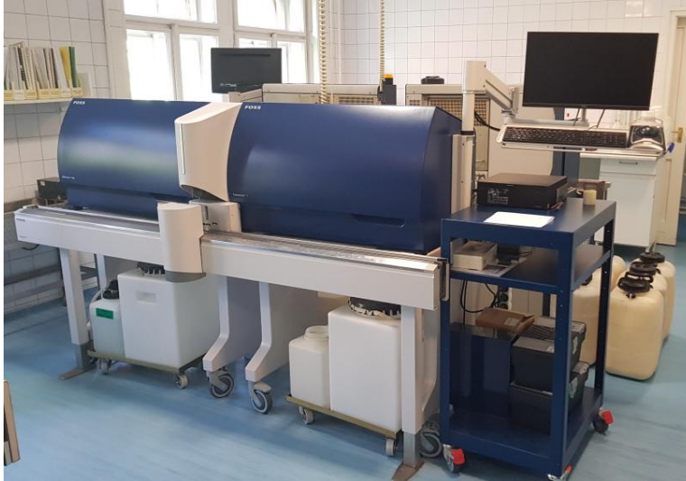
Figure 3: The Fossomatic 7 device used by MTKI, which, combined with the MilkoScan device used to test the content parameters of raw milk, forms the CombiFoss instrument.
